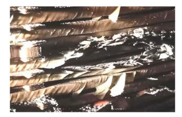
After that, the line auto-reclosed after one second. The auto reclosure was also successful. However, GT tripped on its internal fault while supplying a short circuit current to the line fault. Subsequently, when GT was inspected in the vendor's presence, extensive deformation of windings was observed.
