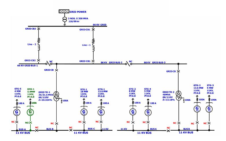
This Plant experienced back to back faults in GTG 1 and GTG 2, Generator Main field excitation winding. The question being discussed in this Case Study-2 are;
